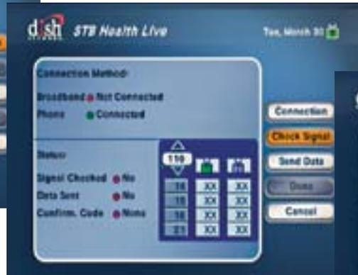
5. Once the connection test is completed, select 'Check Signal' to run the signal test. The 'Testing...' message will be displayed at the bottom of the screen.
