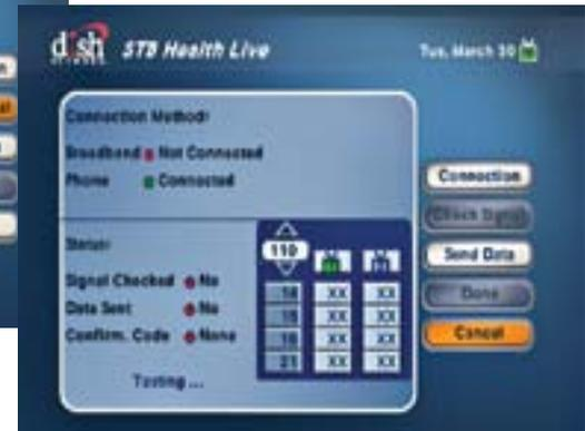
6. This portion of the test runs through the transponders similar to a check switch, a message at the bottom will show the progress.
